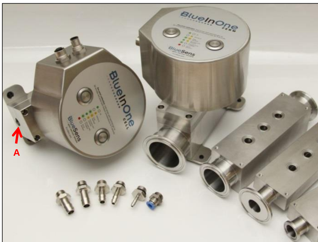
Fig. 5: The various connection options for hoses. The drill hole in the flow adapter (A) has a 1/4" thread. The flow adapter can be exchanged allowing for threads of up to 1 1/4" to be used. Other constructions can be manufactured on request.
